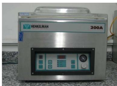
Fig 1. Modified atmosphere packaging (Model: Boxer-200A)
